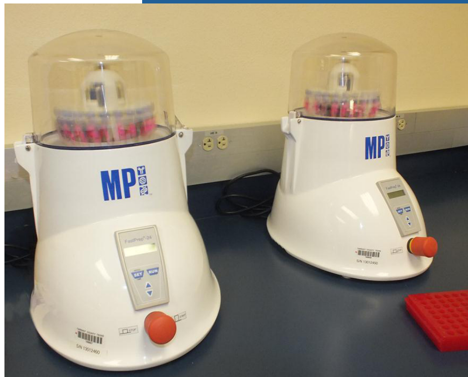
MP Biomedical Fast Prep 24 Homogenizer machines used for liquefying multiple samples of mosquitoes for further viral testing.
